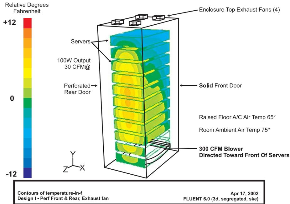
High-powered fans either blowing air into the bottom of a cabinet or pulling air through from the top of the cabinet are not consistent with the principles discussed in this paper. For example, such fans will typically push or pull cooled air through both the front and back of the cabinet, thereby cooling exhaust air (return air), reducing the temperature differential between source air and return air and decreasing CRAC efficiency.
