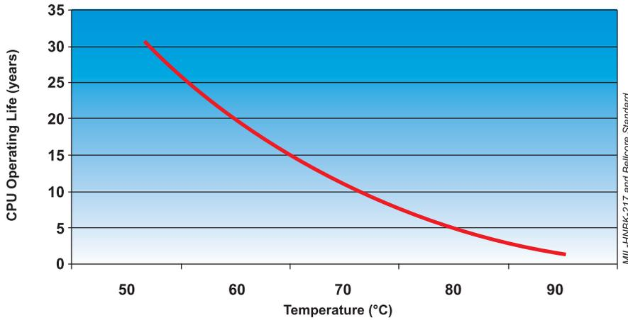
Temperature also effects clock speed. For a 1500 MHz CPU, every 10°C temperature reduction results in a 2% increase in clock speed. While 2% may not seem particularly significant, in a larger data center dedicated to processing large numbers of transactions with 2 RMU servers, losing that extra 2% of transaction turnover means having to buy and install an otherwise unnecessary server every two and-a-half racks.
