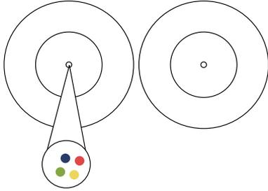
**WDM technology using different color wavelengths of light on a single fiber (40GBASE-LR4, 100GBASE-LR4, and 100GBASE-ER4)**
