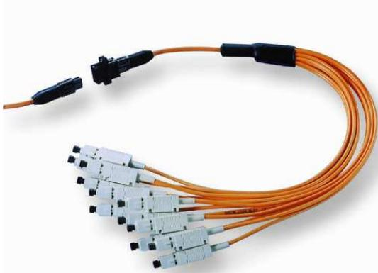
Fan-out cable assemblies offer option for bypassing patch panels. Using an MPO coupler, a trunk cable MPO connector can be mated to an MPO fan-out assembly, which is terminated in MT-RJ, LC, ST, or SC connectors. This option works best with cabinets or with MPO patch panels, but may reduce the flexibility of future modifications to the cabling infrastructure.
