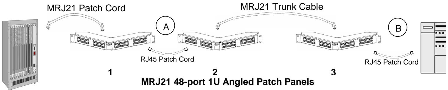
A third example, this one using the MRJ21 platform as an extension of the switch face, is similar to traditional RJ21 breakouts with the MRJ21 benefits of higher density and improved cabling efficiencies. This model also enables the easy migration to MRJ21-based equipment with the
