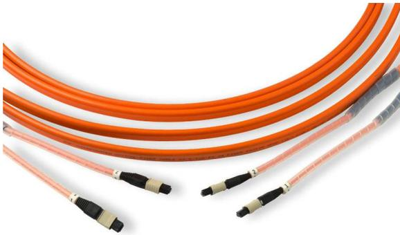
Trunk cables are pre-terminated at the factory with high-density MPO connectors. Each MPO connector terminates 12 optical fibers in a single, push-pull connector about the same size as one SC or ST-style connector. The high fiber density of this connector means that a terminated cable can be placed into cable trays or even pulled in conduit without requiring
