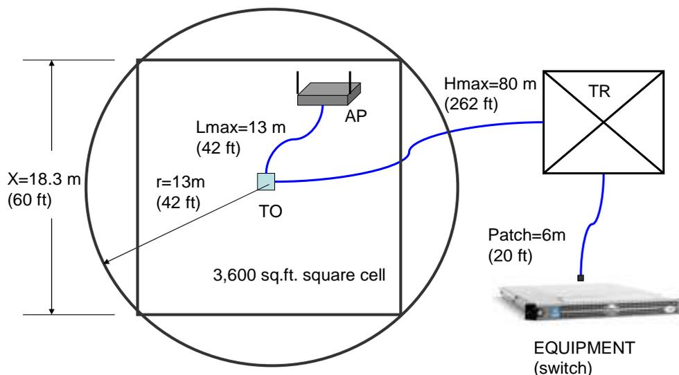
Figure 2- Wireless access point installation in a 60' x 60' building cell
