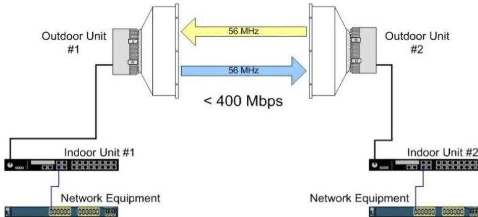
**Figure 2 - Single RF Channel Configuration, Split Mount**
