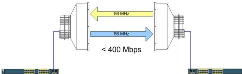
**Figure 3 - Single RF Channel Configuration, All-Outdoor**
