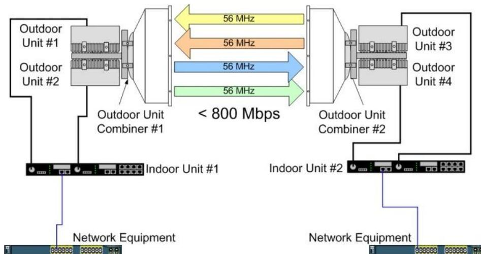
Figure 5 - Dual RF Channel Configuration, Implementation "B"
