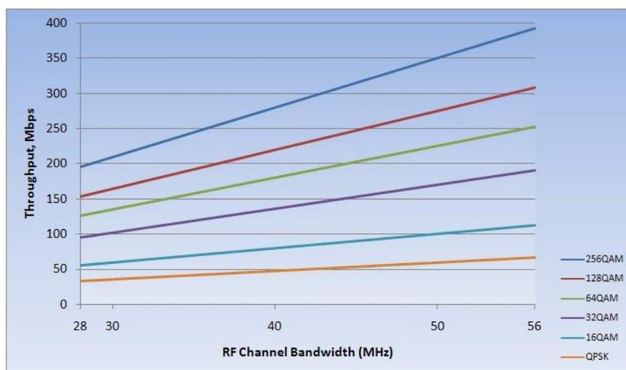
*Figure 1 - Throughput vs. RF Channel Bandwidth*
