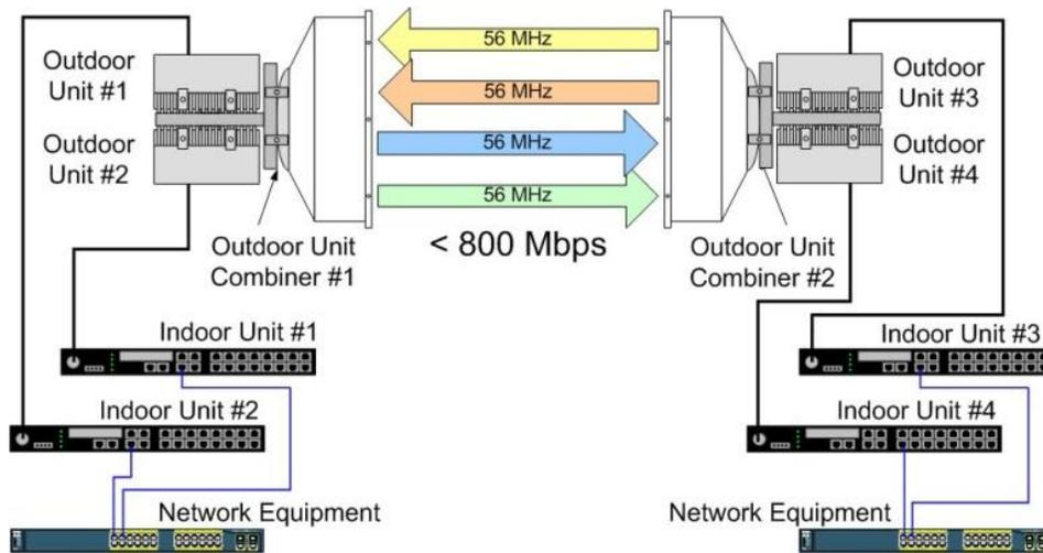
Figure 4 - Dual RF Channel Configuration, Implementation "A"
